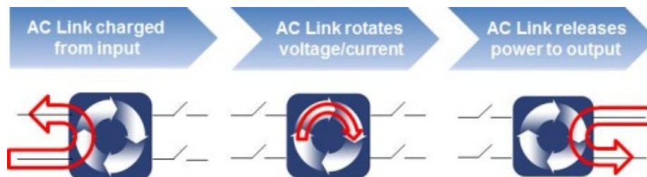
Figure 1: Schematic of PPSA Process
